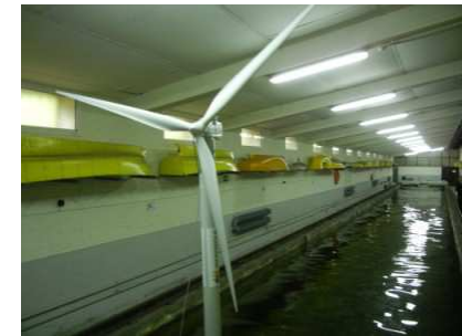
Source: Iberdrola, Testing of Floating foundation at the School of Naval Engineering in Madrid
